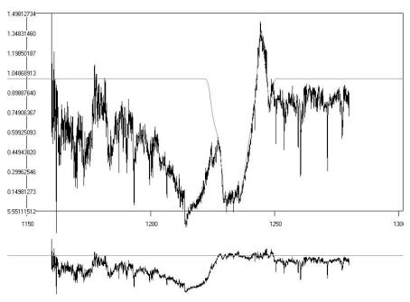
Fig. 2. The N V  $\lambda\lambda$  1238.821, 1242.804 Å resonance lines the spectrum SWP18941 of HD 24912. Each of N V spectral lines consists of three SACs.
